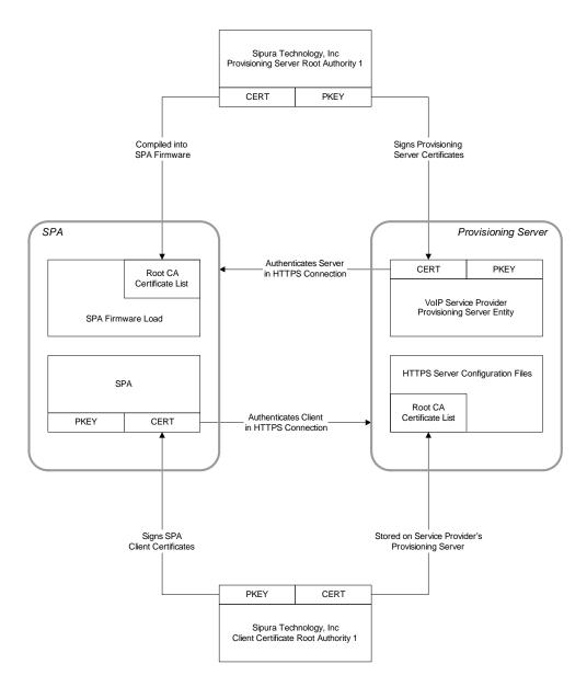
As indicated in the lower half of the diagram, a Linksys Client Certificate Root Authority signs each unique certificate. The corresponding root certificate is made available to service providers for client authentication purposes.
